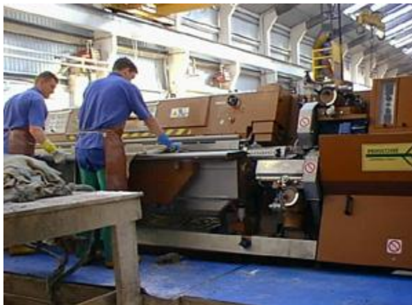
Fig.1-8: Splitting and shaving
