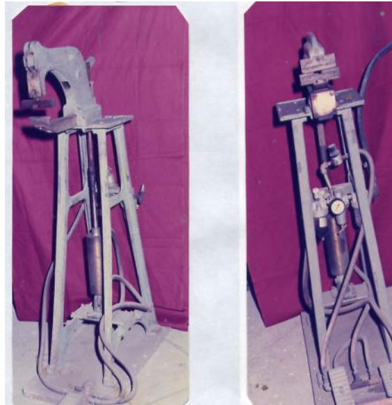
Fig.5-11: Frame opening and closing machine
