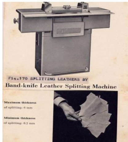
Fig.6-8: Splitting of leather components
